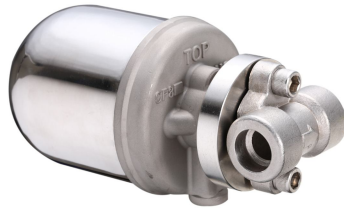
S.S F&T STEAM TRAP No : F77 CONN.SE : 1/2"~1" MAX:590KG/HR 17KG/CM 2
