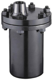
FORGED STEEL & S.S316 IB STEAM TRAP No : 642~946F CONN.SE:1/2"~2" MAX:8,600KG/HR 69KG/CM 2
