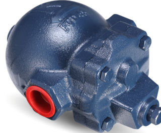
DUCTILE IRON F&T STEAM TRAP No : F22 CONN.SE : 1/2"~1" MAX:590KG/HR 17KG/CM 2
