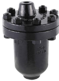
FORGED STEEL & S.S316 IB STEAM TRAP No : 941 & 941F CONN.SE:1/2"~1" MAX:400KG/HR 69KG/CM 2
